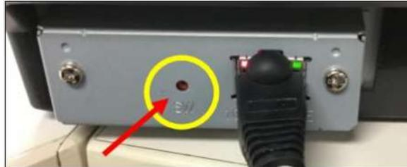
4. With a small screwdriver or pin, you will press the "SW" button until both the NIC LED lights start blinking, then let go of the "SW" button. Both NIC LED lights will be solid.
